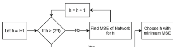
Fig. 2 Flowchart for optimal network architecture selection
